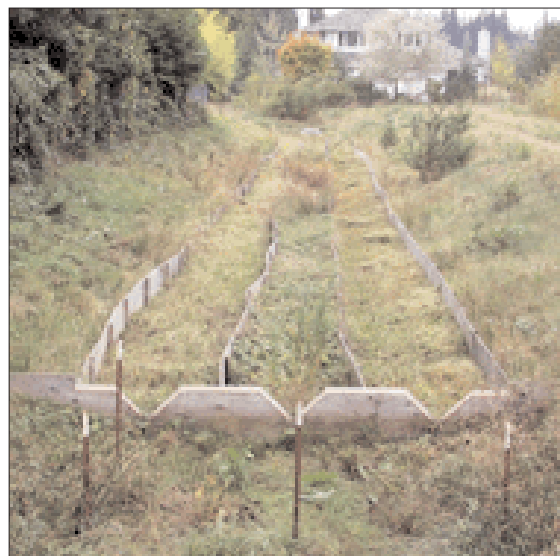
Wet swale with weirs to conduct flow research (Photo: Center for Water and Watershed Studies)
