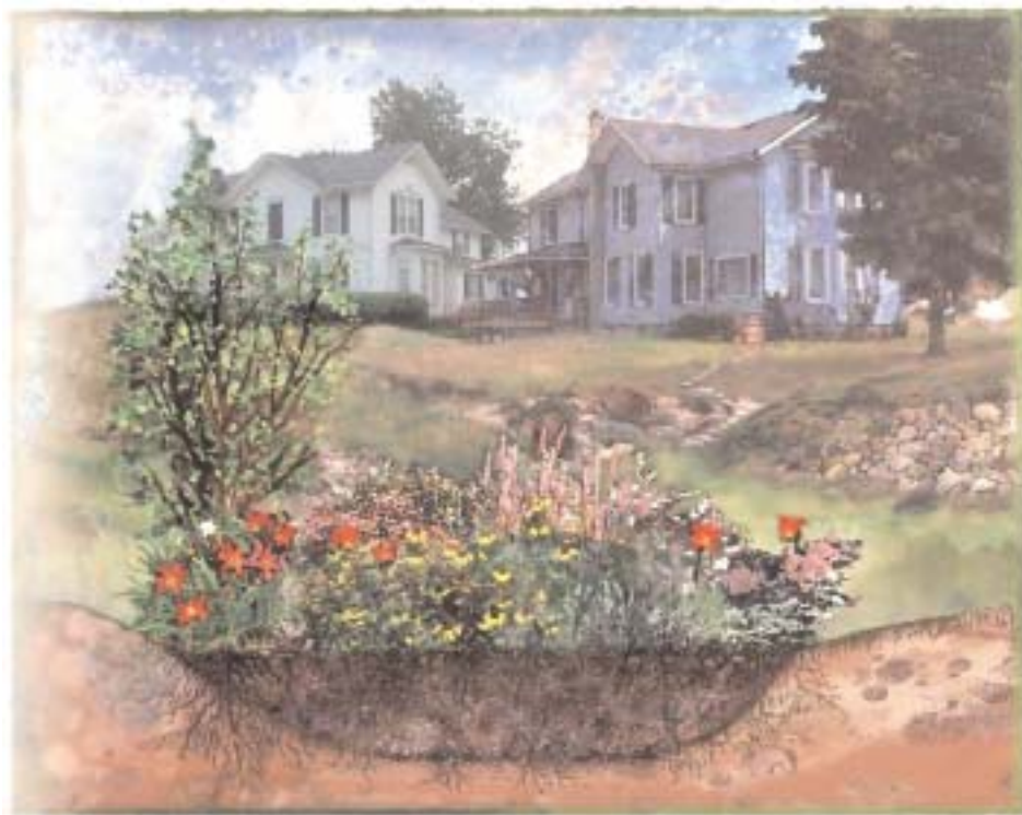
A typical rain garden below the soil (Painting by Ruth Zachary, permission to use by Rain Gardens of Western Michigan)
